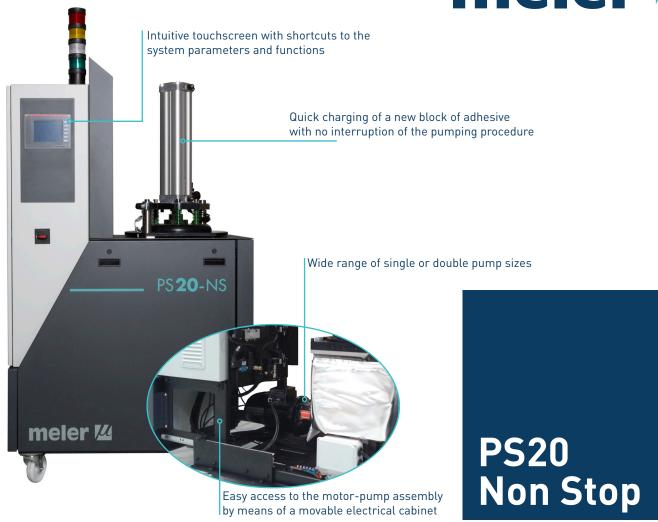
Melter designed to melt 20 kg blocks of PUR. Controlled melting rate. Only melts the adhesive that will be used. The new block of adhesive can be inserted without stopping the unit and, therefore, the production (non-stop system).
